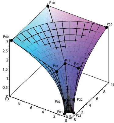
Figure 1: Catenoid patch and its control net with respect to the normalized B-basis of  $T_2 \otimes H_3$ .
